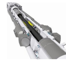
Riserless Drilling Phase 1 (Active RCD)
